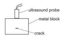
The times between the emission of the ultrasound pulse and the return of the reflections to the probe, and the strengths of the reflected pulses, are measured. The results are shown on the graph.
